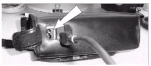
Open the flap on the rear of the MFK 16 to expose the mains power socket. Insert the mains power cable into the socket and plug the other end into a wall socket. <u>The battery is fully charged when the display of the MFK 16 shows "Trickle Charge".</u>
